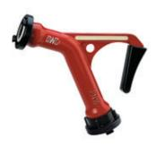
The familiar, comfortable and convenient handling when working with support bends is naturally also possible with our Turbo nozzles and is especially usefully at high pressures and flow rates of 400 l/min and higher. The kickback forces are dissipated downwards via the pressurised hose assembly. The branchpipe operator is therefore largely relieved of the kickback and can work without large exertion and without tiring. The support bend is equipped with a persistent fluorescent liner.
